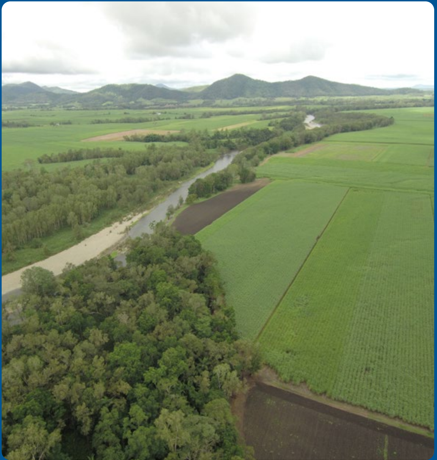
Figure 24: Aerial view of riparian restoration works involving converting sugarcane cropping land to stabilise the bank to mitigate ongoing intensive erosion of prime cropping land. Photo credit: Reef Catchments
