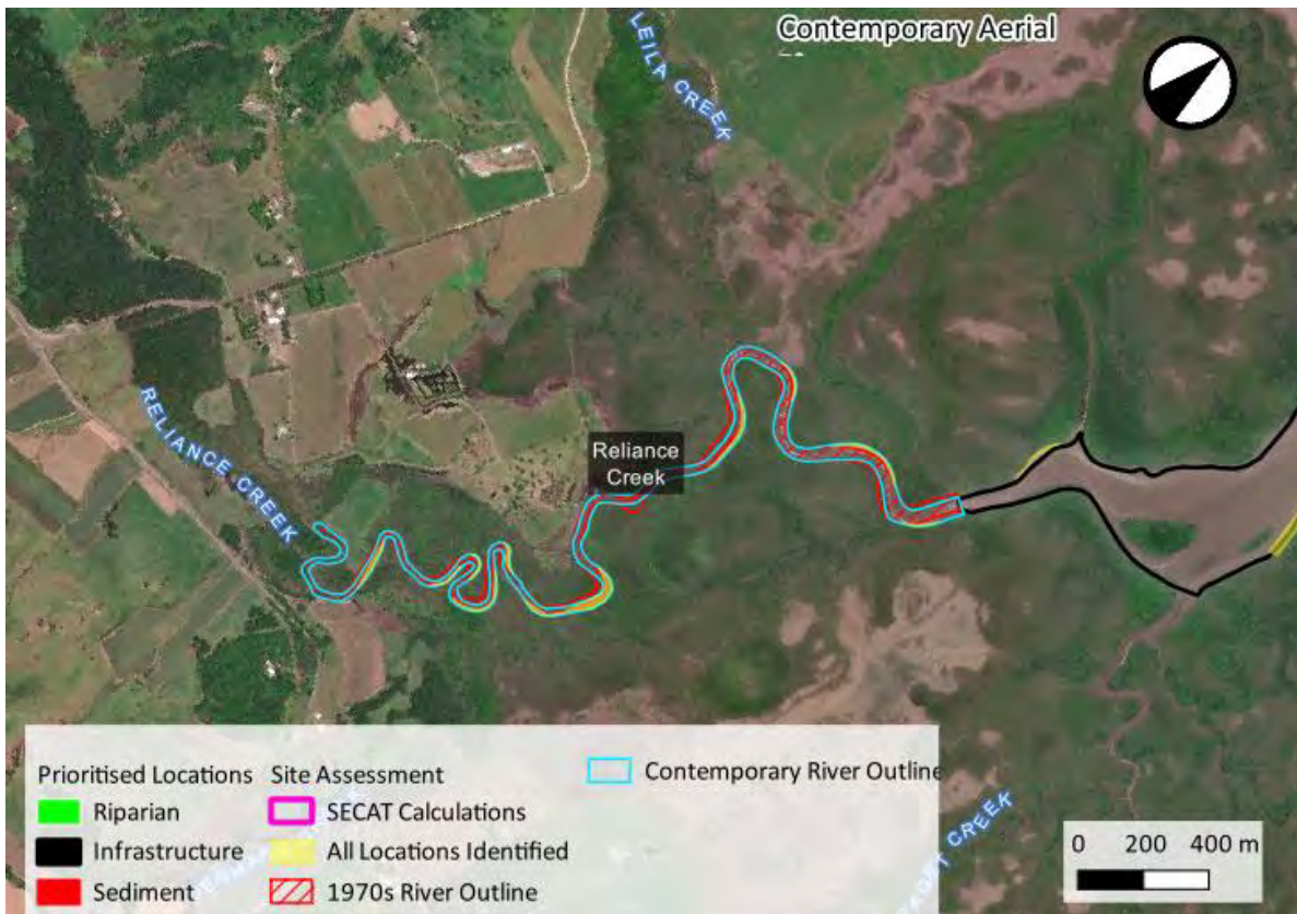
Figure 71. Bank traces between 1970s and present with locations of recent movement highlighted
