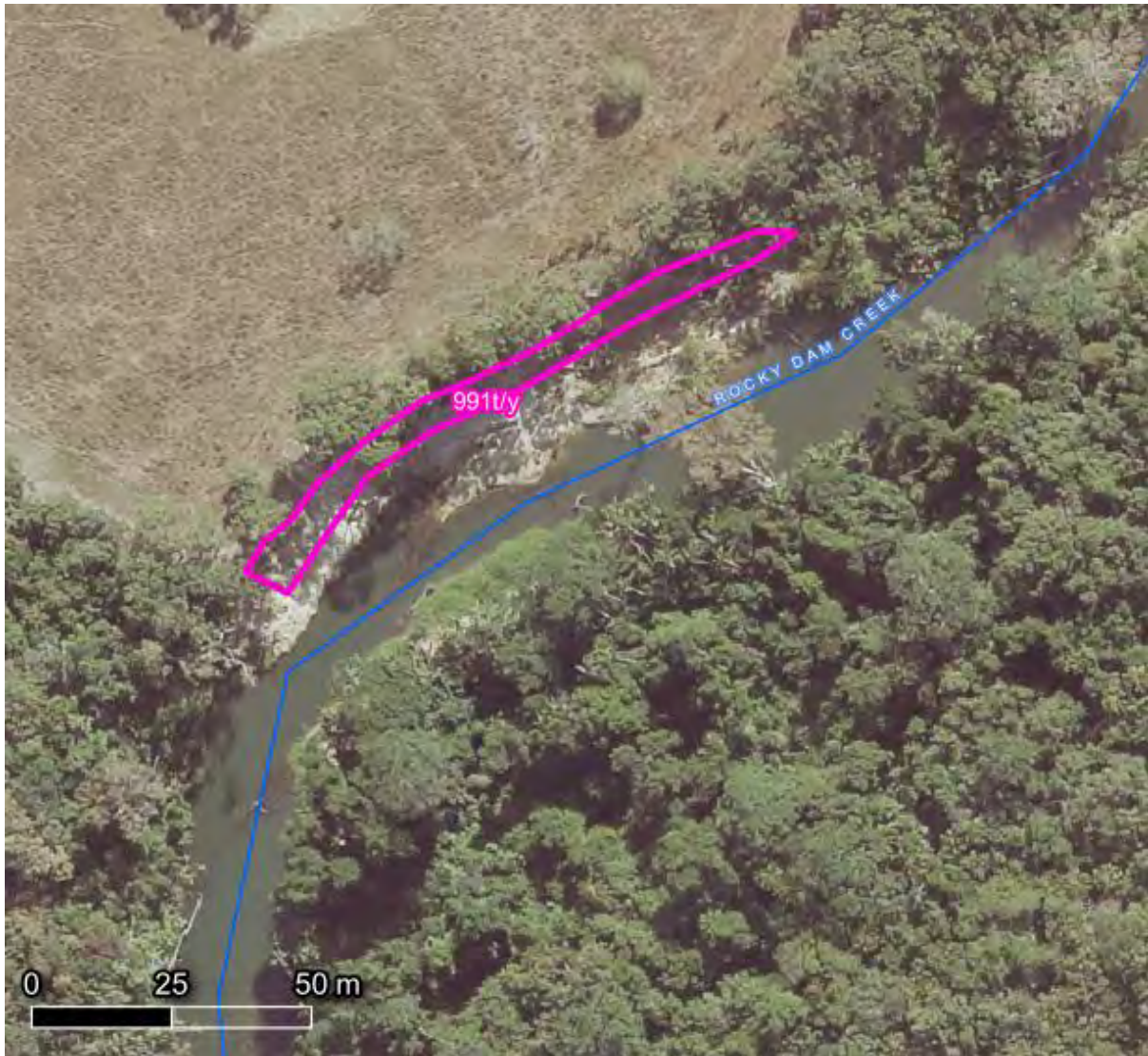
Figure 96. Close up aerial of Site 336, a near-vertical 12m high bank on Rocky Dam Creek
