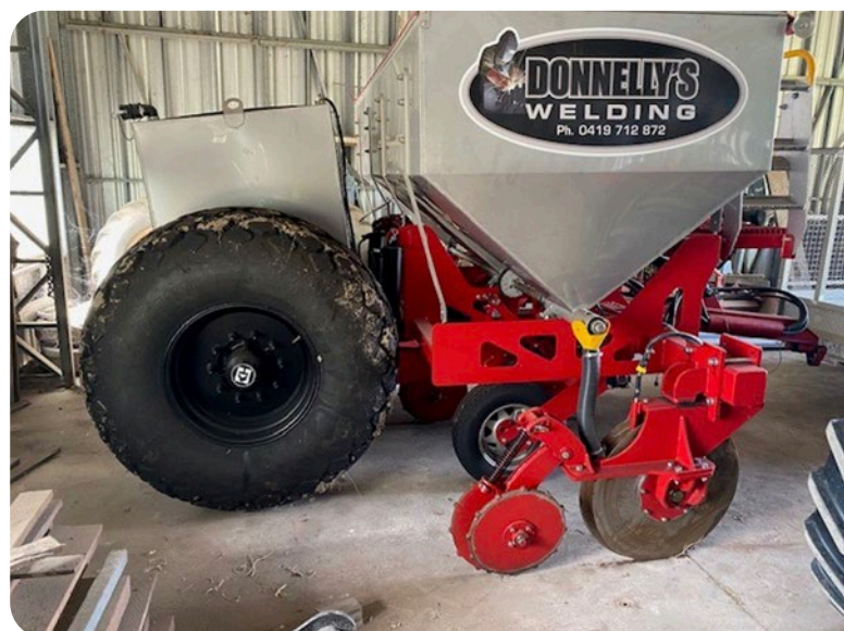
Figure 1: Stool splitter fabricated by Donnelly's Welding
