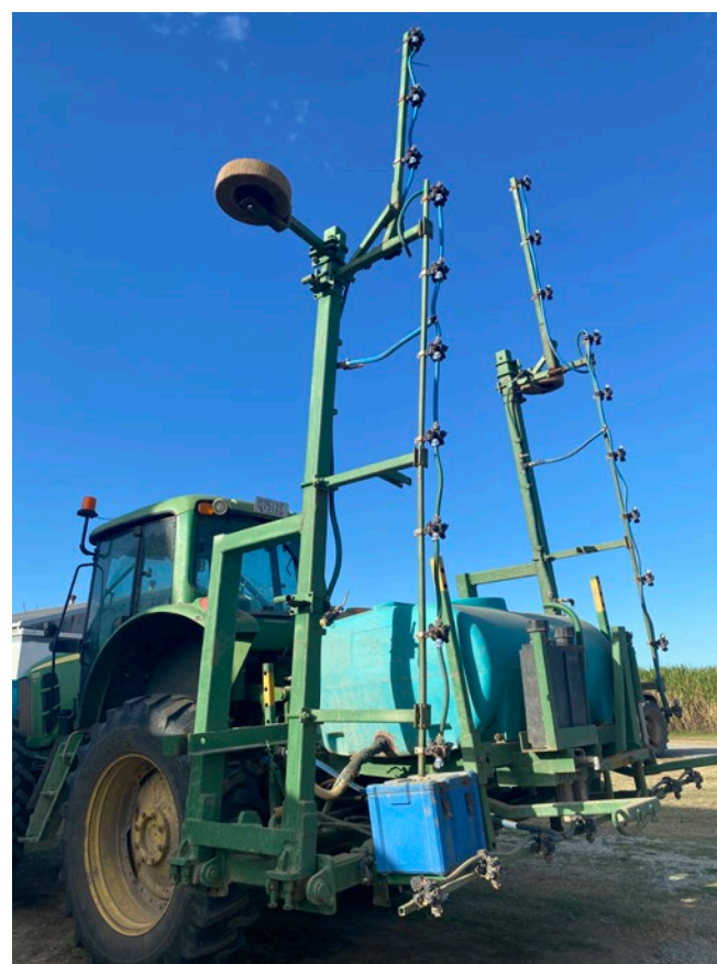
Figure 2: The boom that was assessed by Adam Keilbach, Senior Field Officer at Farmacist Mackay, and upgraded through funding with plumbing, fittings and nozzles. Photo by Che Trendell, Farmacist.
