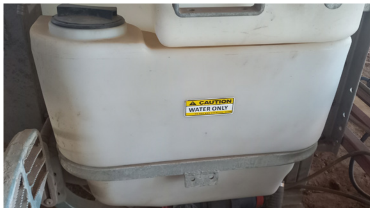
Figure 3: The new spray tank in conjunction with the flow rate and section controller have improved the efficiency of chemical applications. Photo by Che Trendell, Farmacist.
