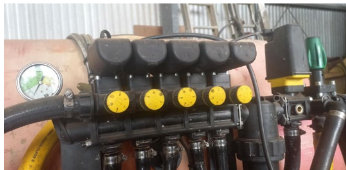
Figure 3: Flow rate controller installed on the Anderson's spray rig as part of Project OASIS funding.
