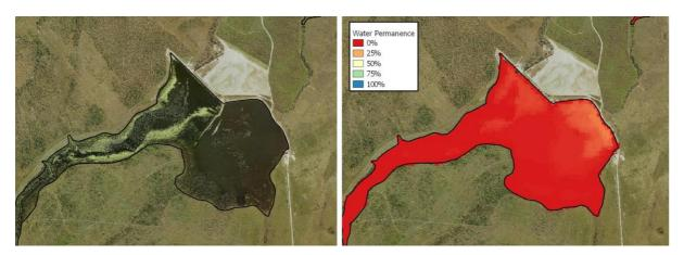
Figure 24. WOFS returning a low water permanence signature despite the substantial amount of deep water in this irrigation dam. Review of historic images revealed this dam was constructed in 2016, a relatively short period compared to the 36 years of imagery used for the time series.
