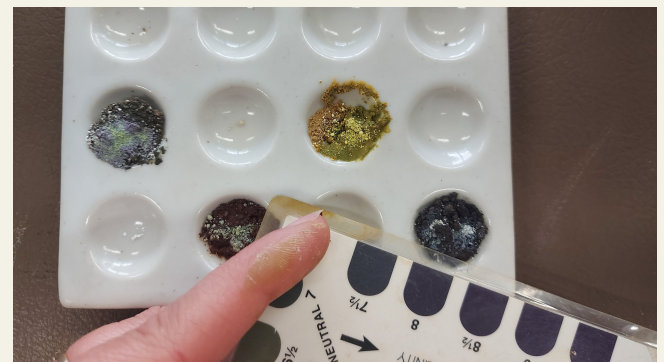
Figure 1: Carrying out a soil pH test. Compare the colour to the test card to estimate the soil pH.
