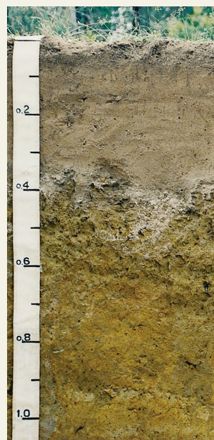
Image 4: Texture contrast soils have a sandier/light textured topsoil which overlies a clay/heavy textured subsoil (which is usually sodic and/or saline).
