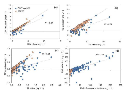
**Figure 5.** Correlations between (a) DIN, (b) TN, (c) TP, and (d) TSS reduction in concentration (mg L<sup>-1</sup>) and inflow concentrations in constructed treatment wetlands (CW), vegetated drains (VD) and sewage treatment plant wetlands (STPW) in tropical and subtropical Australia. Correlations are for all treatment wetlands aggregated and are significant (*p* < 0.001).
