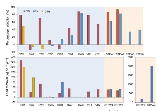
**Figure 3.** Nitrogen (DIN, TN, and TDN) removal (% and kg ha<sup>-1</sup> yr<sup>-1</sup>) by constructed treatment wetlands (CW), vegetated drains (VD) and sewage treatment plant wetlands (STPW) in tropical and subtropical Australia. Values are mean  $\pm$  standard error.
