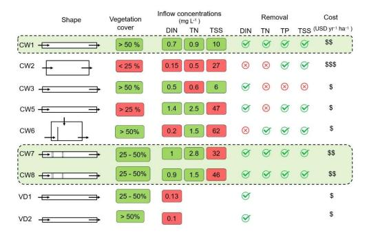
**Figure 7.** Summary of parameters associated with efficient DIN, TN, TP, and TSS removal and cost (APVC, annualised present value cost) of constructed treatment wetlands (CW) and vegetated drains (VD) in tropical Australia. Sites with a tick mark are those where removal was observed. = <USD 5000; = >USD 5000 <USD 10,000; = >USD 10,000.
