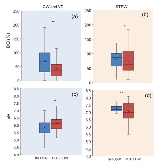
**Figure 4.** Difference between the inflow (blue) and outflow (red) in pH and dissolved oxygen (DO%) for (**a**,**c**) constructed treatment wetlands (CW) and vegetated drains (VD) and (**b**,**d**) for sewage treatment plant wetlands (STPW). Significant differences between the inflow and outflow are shown as \* p < 0.05 and \*\* p < 0.001.
