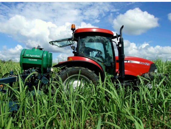
Shielded spray unit to distribute pesticide directly where it is needed
