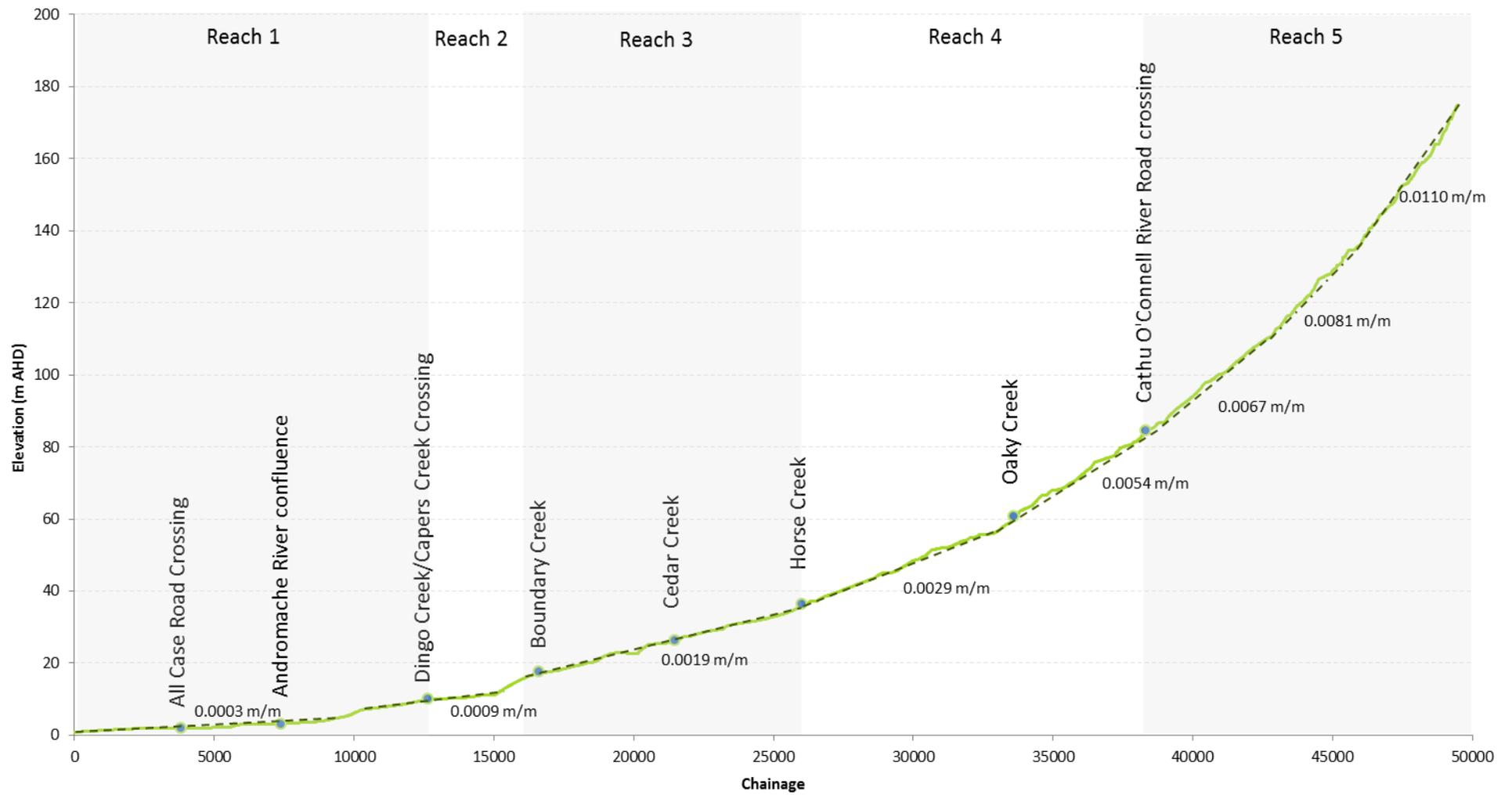
Figure 8. Longitudinal bed grade along the O'Connell River.
