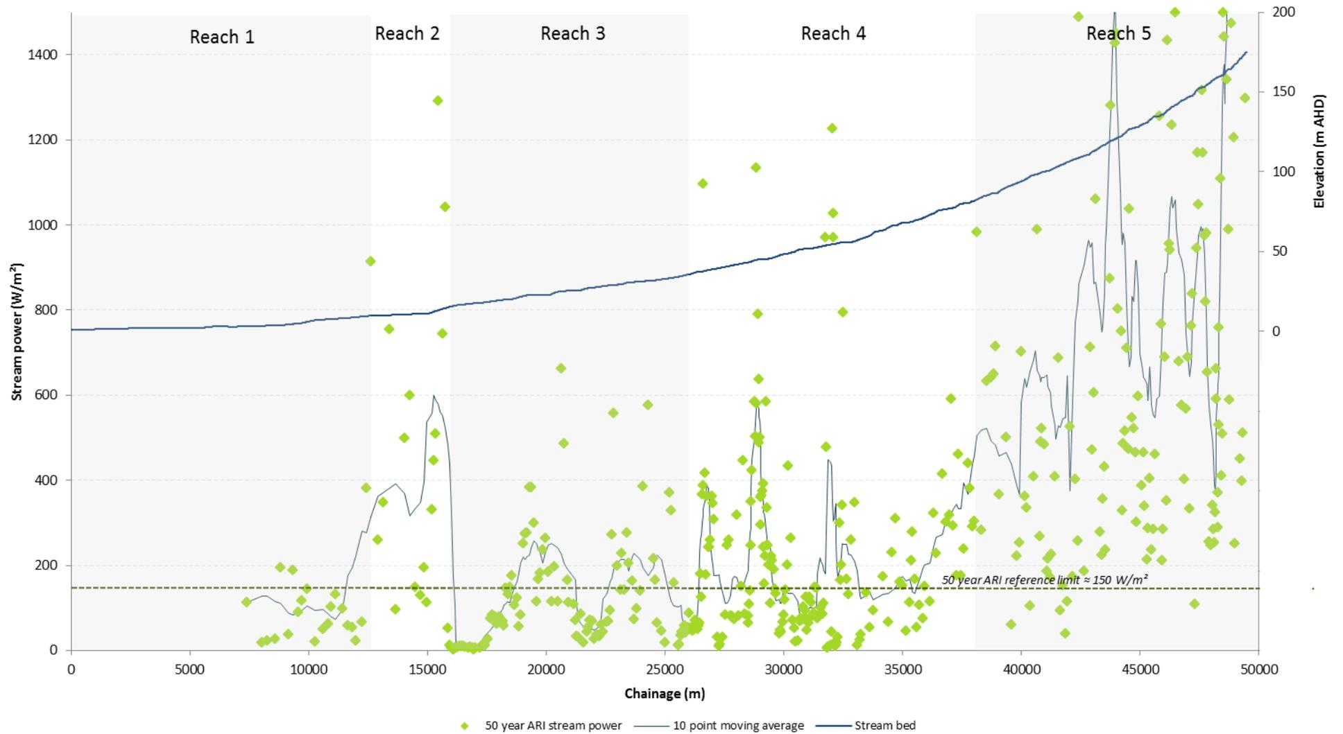
**Figure 10 . Results from the fifty year ARI stream power assessment along the O'Connell River along with the reference value - hydraulic model only extend upstream of the Andromache confluence**
