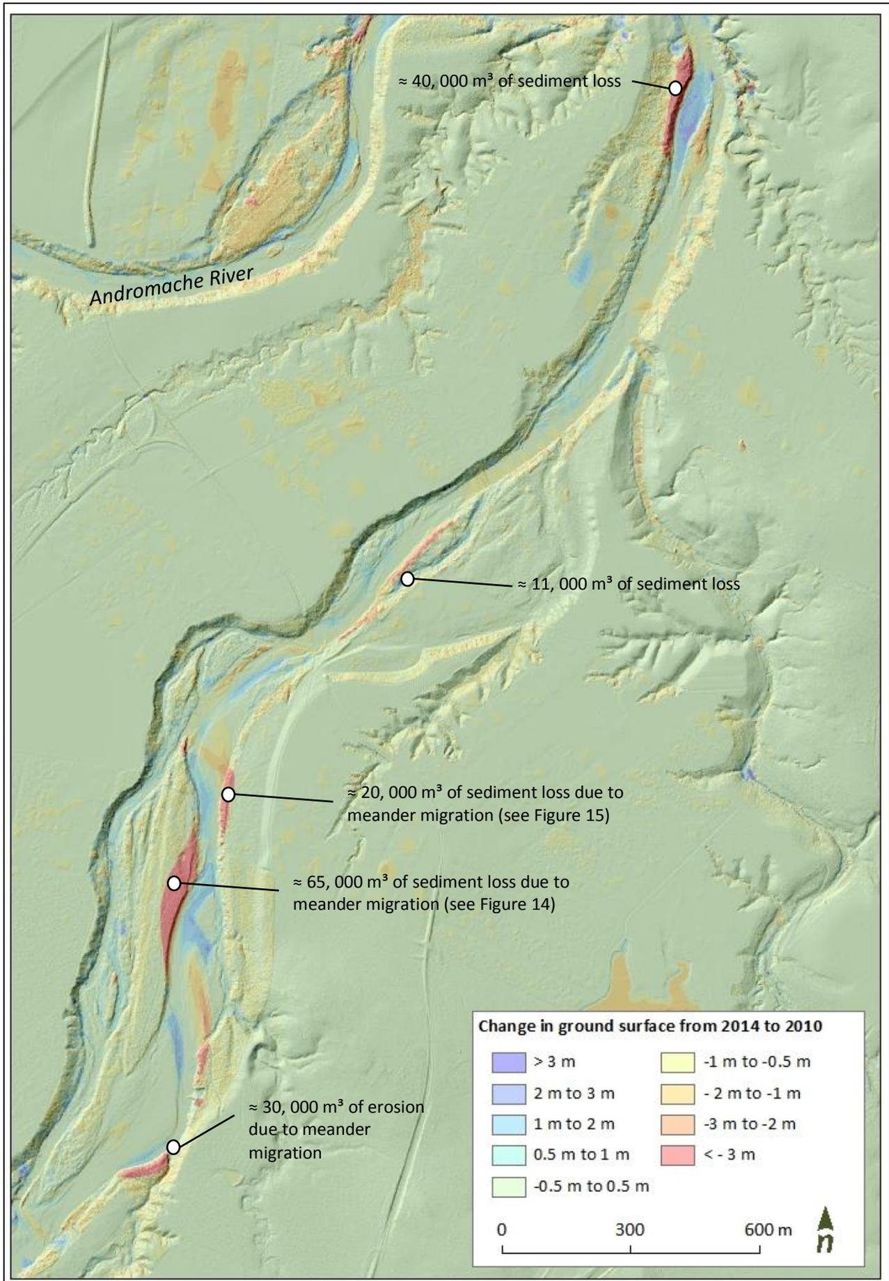
**Figure 13.** Changes in elevation between 2014 and 2010 included estimates of sediment loss in the area upstream of the Andromache River confluence.
