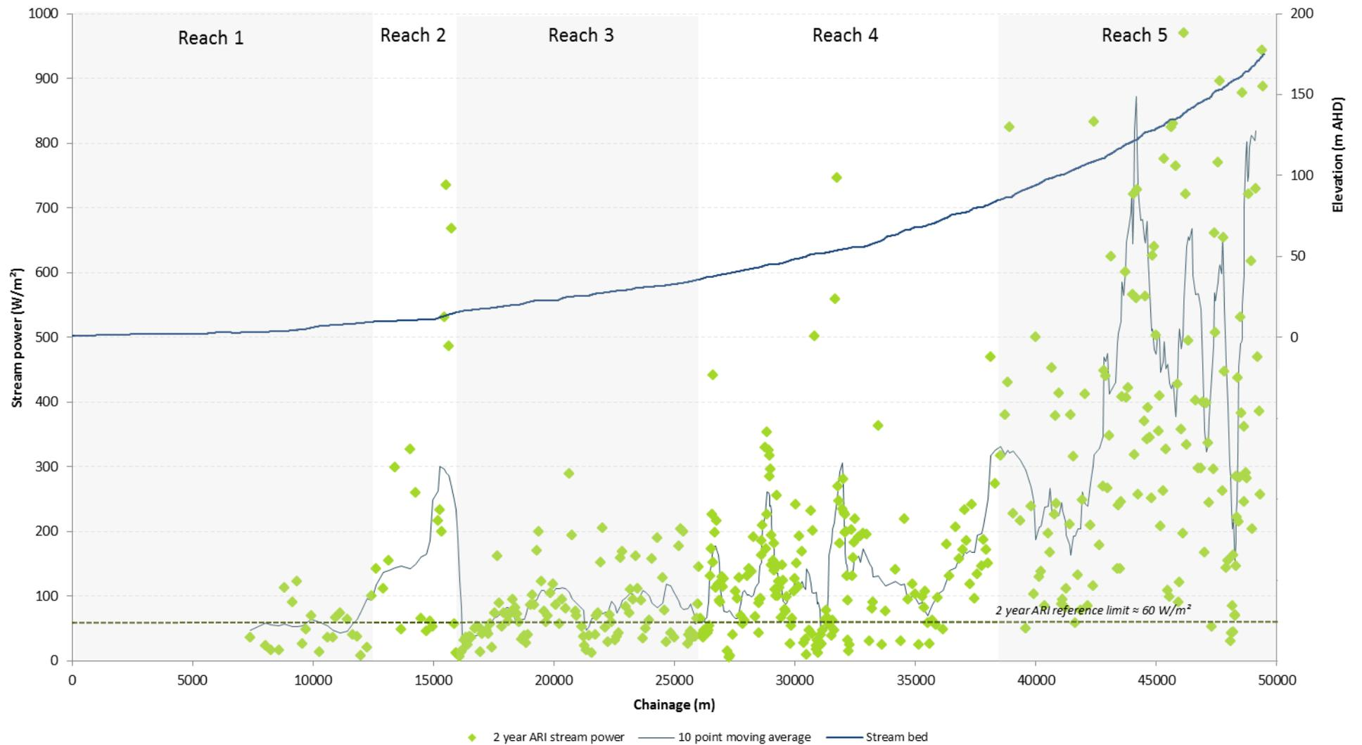
**Figure 9.** Results from the two year ARI stream power assessment along the O'Connell River along with the reference value – hydraulic model only extend upstream of the Andromache confluence
