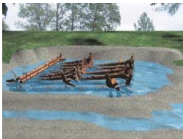
Step 8. Place a pair of cross spanning logs at the downstream end of the structure.
