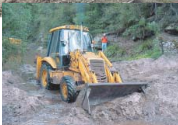
Photo 39. A 4WD tractor/loader like this one is an essential piece of equipment at a log structure construction site. It can be used for moving logs around on site, backfilling structures and regrading the site.
