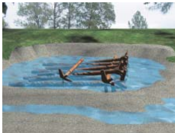
Step 6. Place a second cross spanning log.
