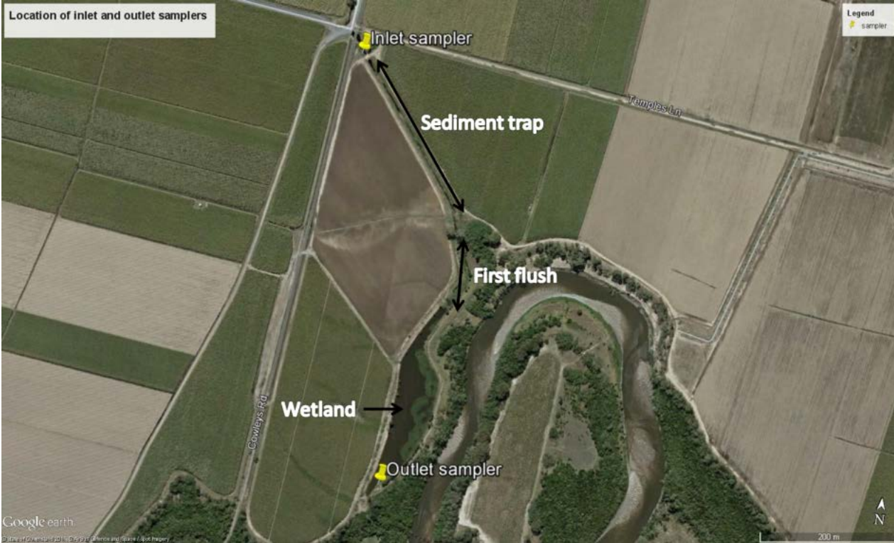
Figure 2 The three components of the system repair site, and the location of the water quality samplers
