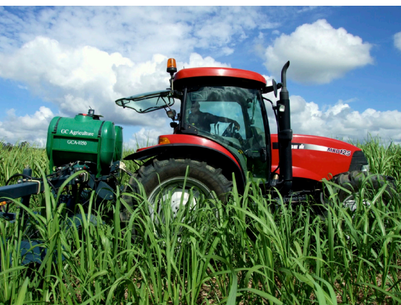
Shielded spray unit to distribute pesticide directly where it is needed
