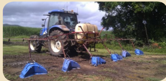
ABOVE: Shielded spray units allow growers to use knockdown herbicides in the inter-row and reduce reliance on residual herbicides.
