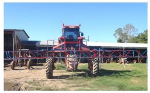
Reef Rescue helped Alligator Creek cane farmer John Simpson install a front mounted spray rig on his high clearance tractor for improved efficiency and precision application of nutrients and chemicals for best water quality management.
