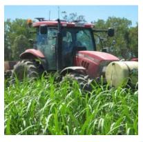
John Deguara's tractor with GPS roof array and front tank carrying shielded sprayer. The GPS variable rate control unit delivers precision nutrient and chemical applications to improve efficiency and accuracy of operation.
