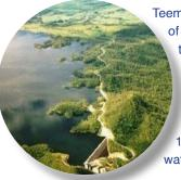
Teemburra Dam 50km west of Mackay occupies the top of the Blacks Creek catchment with a surface area of 1040 hectares, an average depth of 14.2 meters and holds 147,500 mega litres of water at full capacity.
