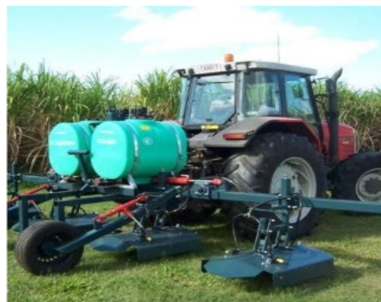
Lou Raiteri's shielded sprayer setup for controlled traffic farming system. The introduction of precision agriculture farming systems yield long term improvement in soil health, along with immediate benefits such as improved moisture retention and weed control.
