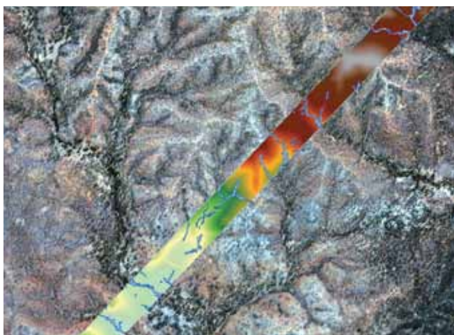
Airborne laser technology is being used to improve our knowledge of gully erosion processes.
