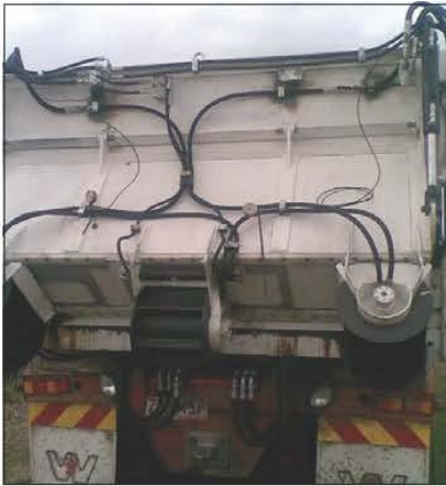
A mill mud truck fitted with side applicators fitted to enable banded application
