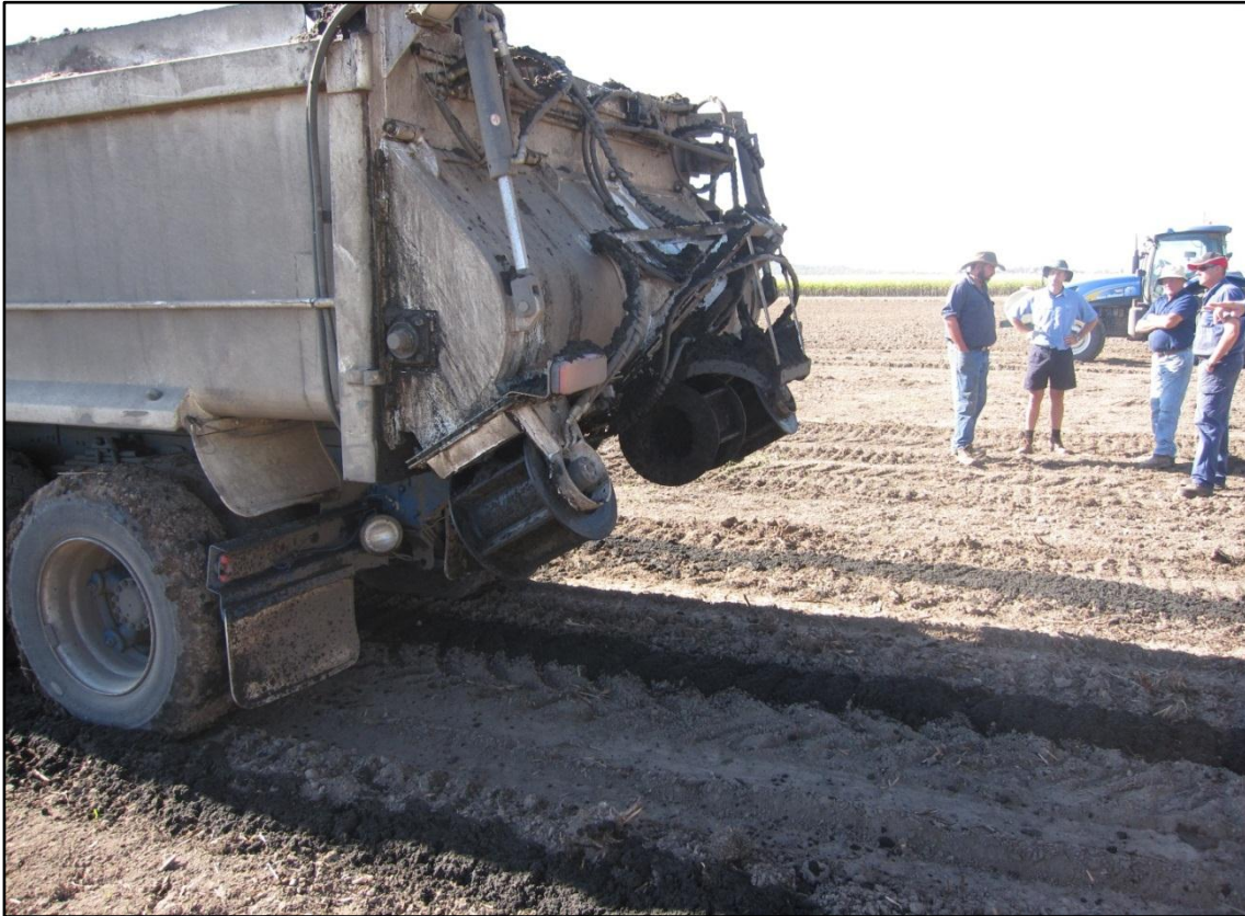
Back of truck Mill Mud spreader which applies mud directly onto the cane row
