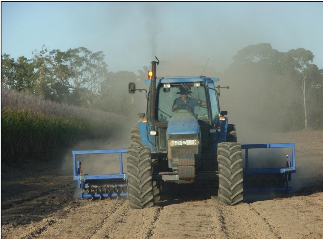
3-row wavy disk cultivator funded through Reef Rescue confines compaction to the inter-row
