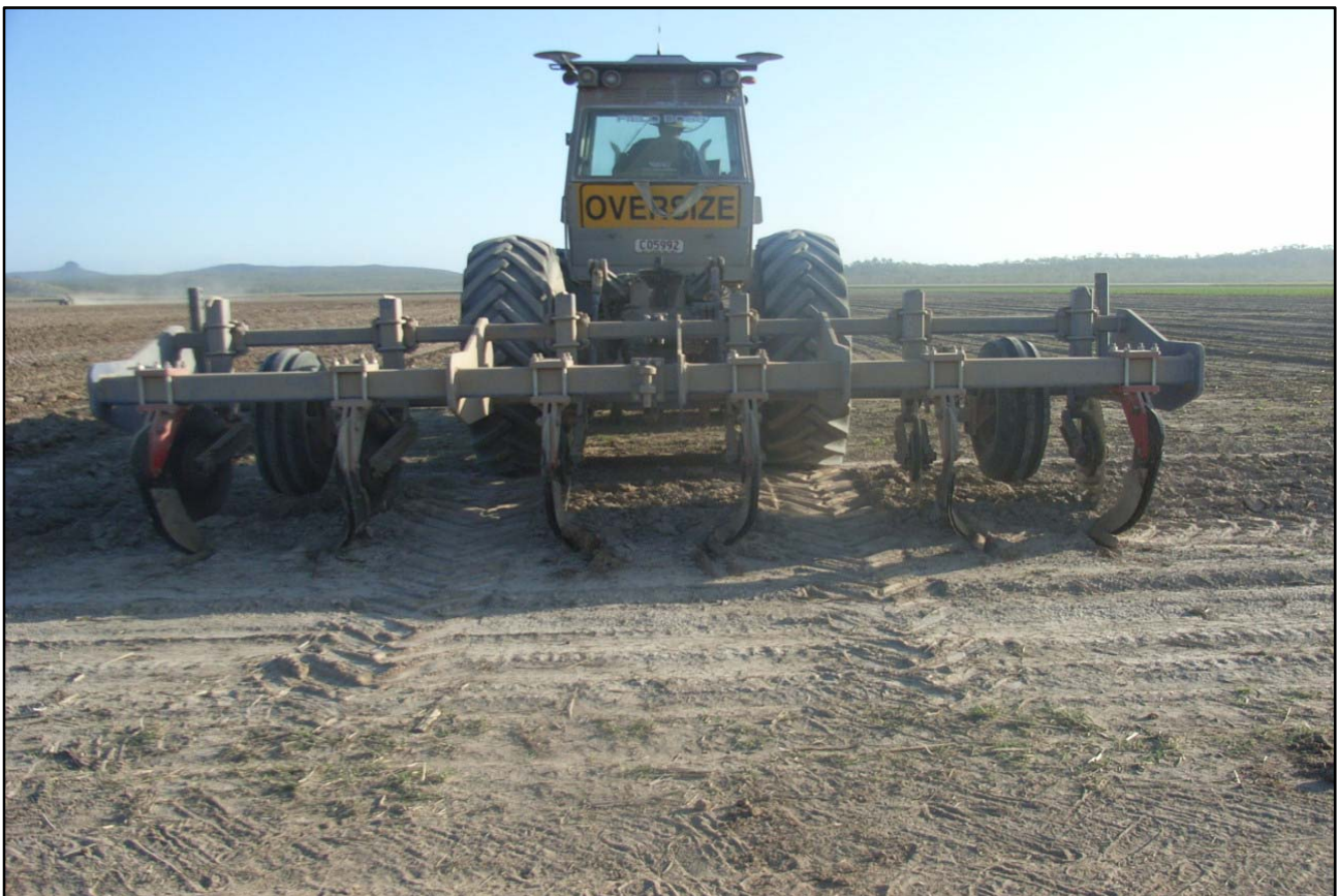
Plate 12 Example of one of the cane projects funded through Reef Rescue is a 3-row zonal ripper and GPS guidance for a controlled traffic zonal tillage system.
