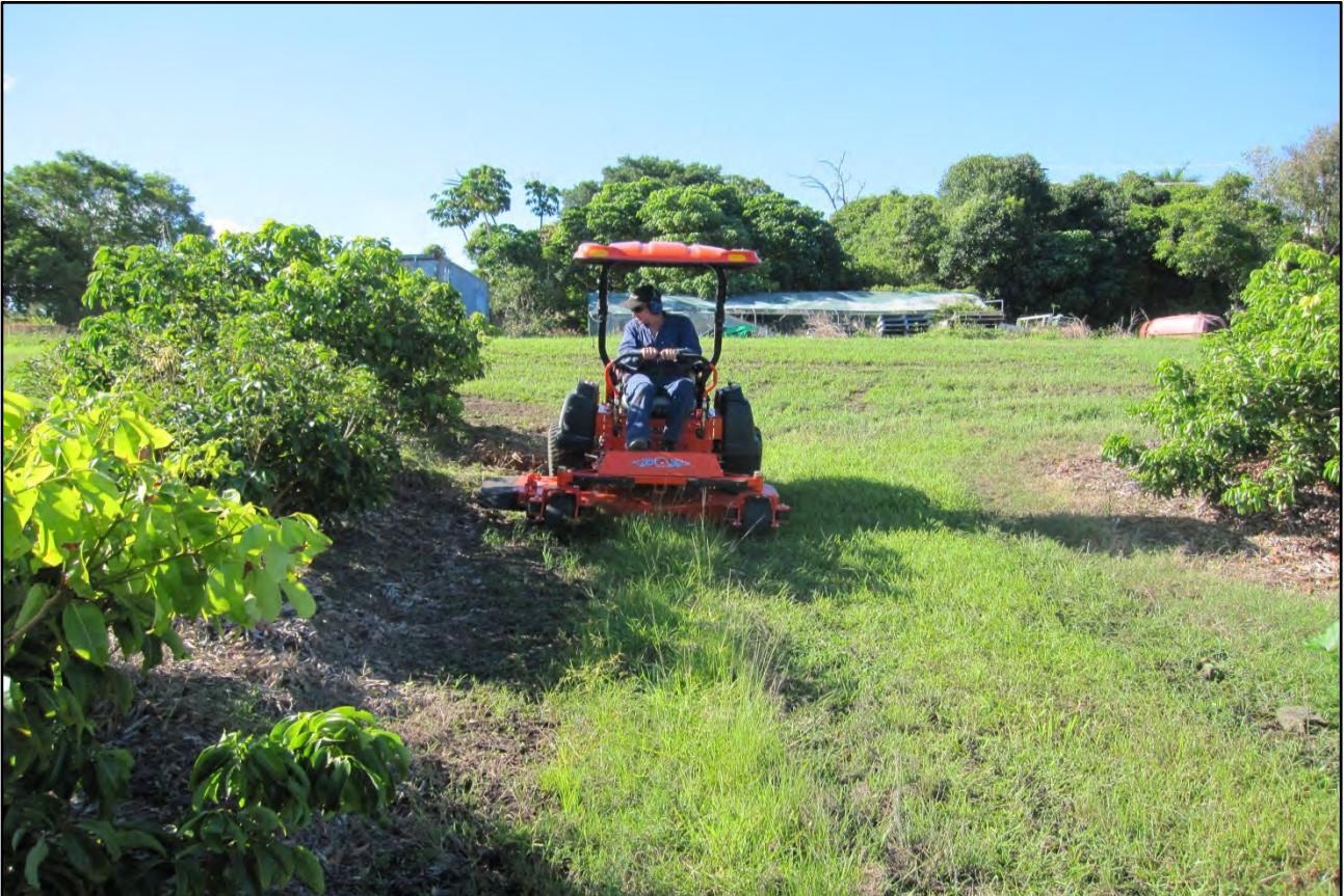
Plate 15 An example of a Reef Rescue funded horticulture project is a side throw mulch mower for maintaining good inter-row ground cover and mulching for weed control.
