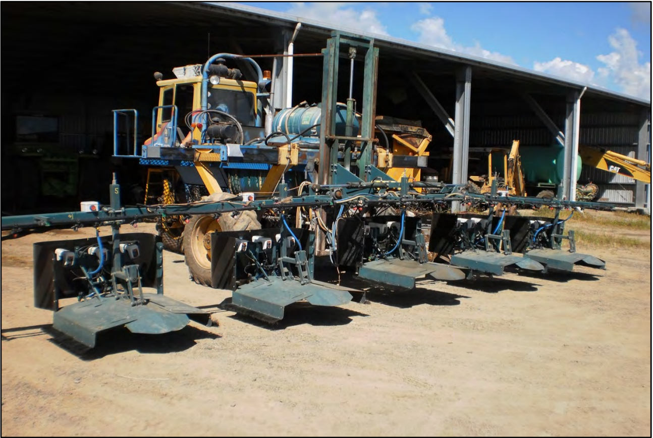
Plate 4 Cane Industry Project looking at WeedSeeker® technology and shielded sprayers
