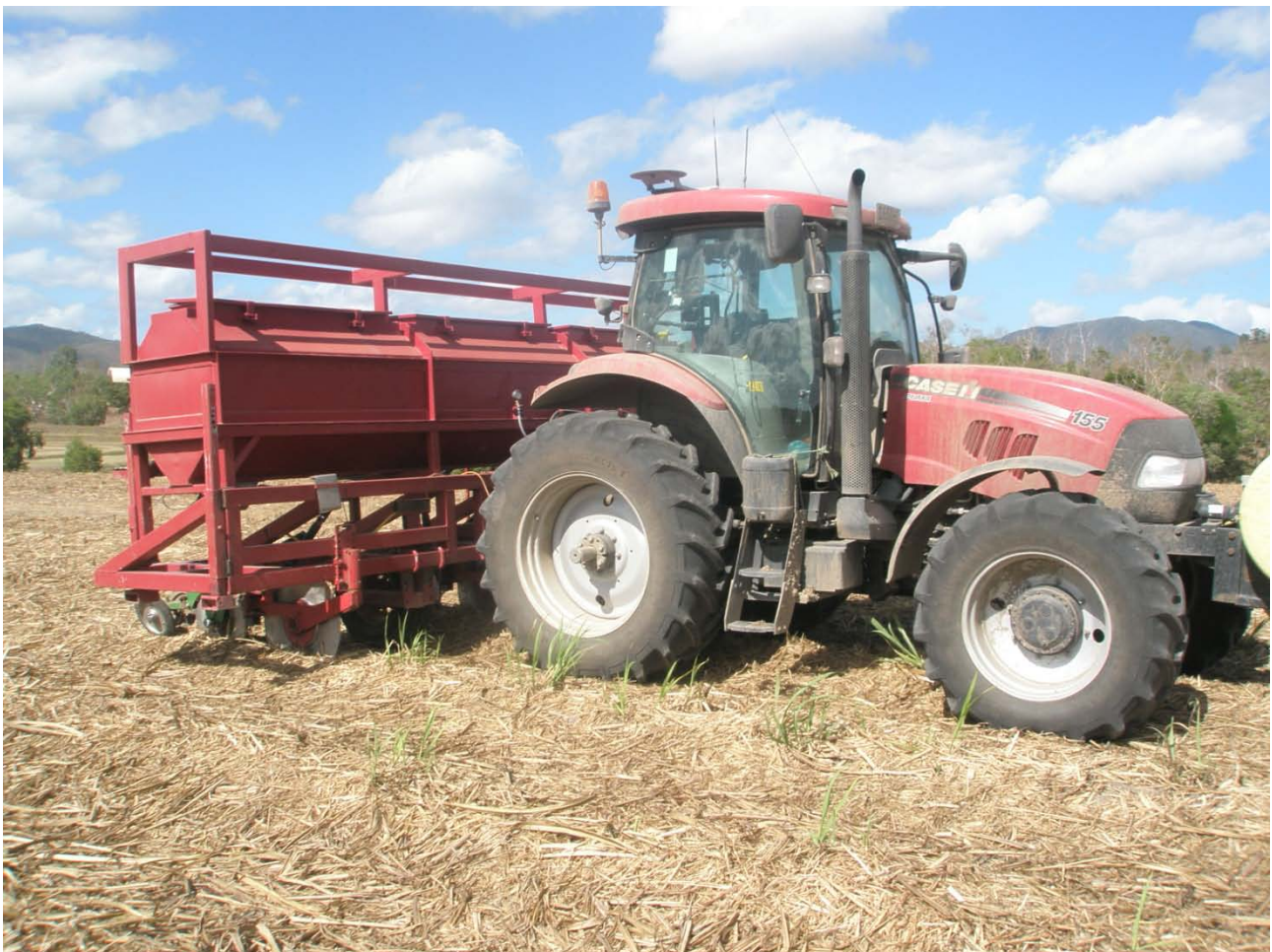
Plate 9 Example of one of cane the cane projects funded through Reef Rescue is a sub surface fertiliser box with a variable rate controller combined with a GPS and a controlled traffic system
