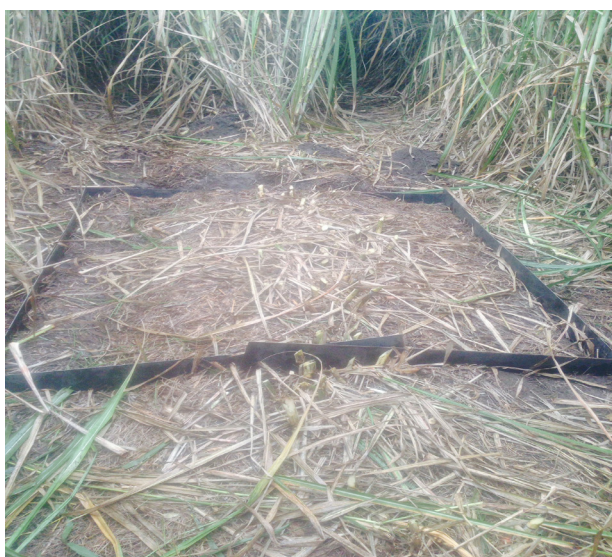
Figure 2 Rainfall simulation plot centred over the cane row (hand cut) and extending to the furrow centres
