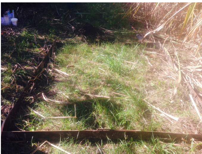
Figure 7 The skip area had less ground cover (than the cane rows) resulting in a higher TSS concentration and load
