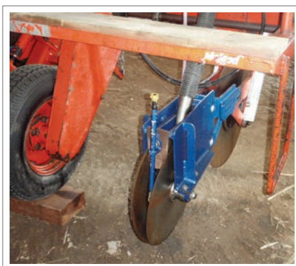
Modifications have been made to this fertiliser box to include double disk openers, which enable fertiliser to be placed below the surface. It's a best management practice which Reef Rescue supports.
